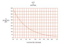
NG Capacitors shall be capable of stable operation with decreased life at 110% of rated voltage at frequencies up to 66 Hz (Sinusoidal) provided the case temperature does not exceed the maximum rated case temperature.
